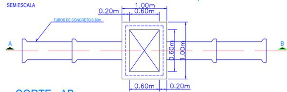
PLANTA BAIXA DA CAIXA DE PASSAGEM (0.60m x 0.60m x 0.50m)
